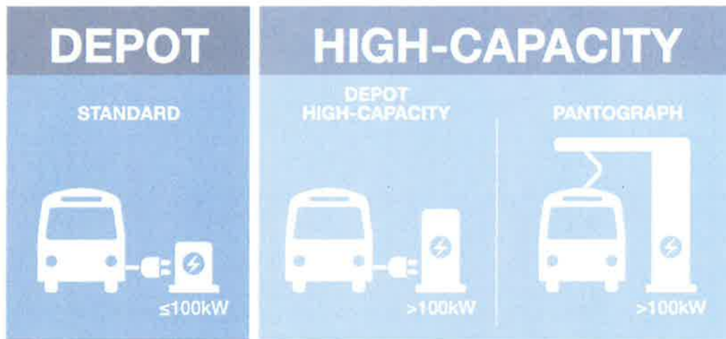
Figure 2. Common Electric Bus Charging Options
