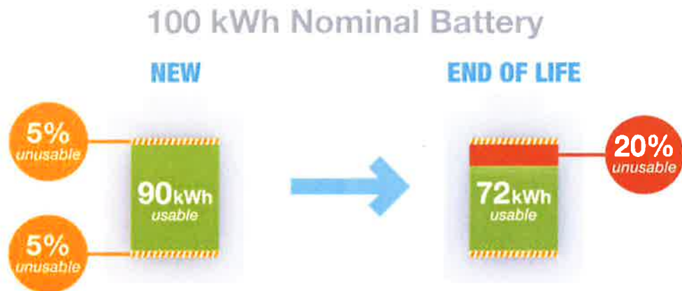
Figure 1. Nominal vs Usable Battery at Beginning and End of Life
